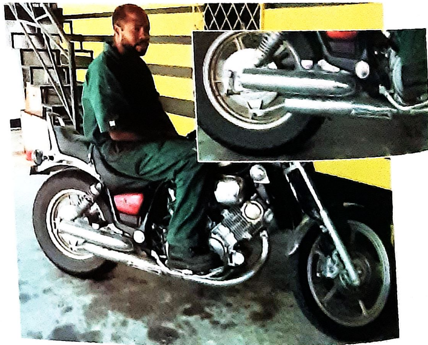
The noise from the engine of a motorcycle is unbearable without a silencer. Inset: Close-up of the silencer
