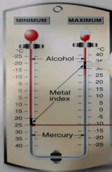
Figure 3.15b A maximum and minimum thermometer
